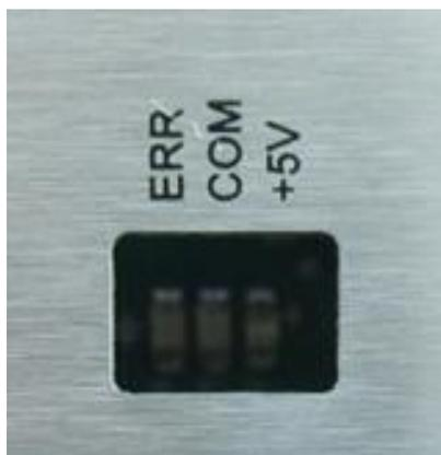
Figure 4: Status LEDs "ERR", "COM" and "+5V" on PiXtend eIO devices
